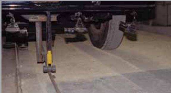
1996 – The lateral confinement function of Tensar geogrids leads to significant reductions in rut depth
