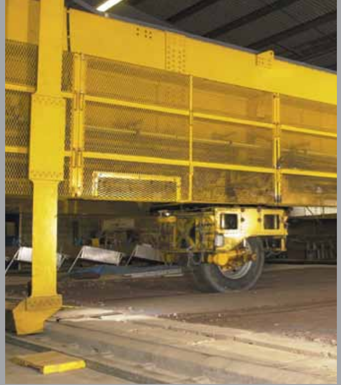
2000 – Full-scale laboratory tests at the UK Transport Research Laboratory comparing Tensar geogrid with alternative forms of geogrid
