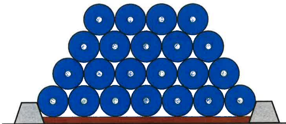
Figure 3. Recommended setup for safe onsite stacked storage of Polyfelt® TM13C High Performance Turf Reinforcement Mat
