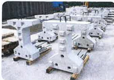
Completed splice blocks
