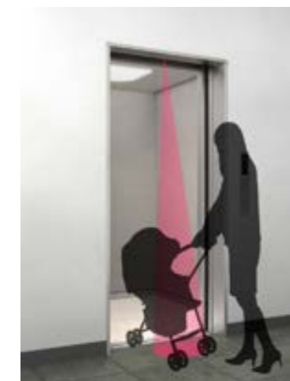
Hall Motion Sensor (HMS) (Optional for CO doors only)
